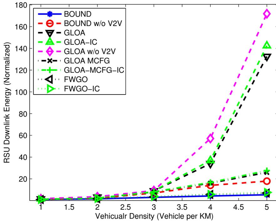
Fig. 6: Total RSU Downlink Energy vs. Vehicular Density (Vehicle per km). The job sizes of all the vehicles are constant and equal to 5 (time slots), and the speed is taken from a Gaussian distribution with a mean 20 m/sec and the standard deviation of 2.
