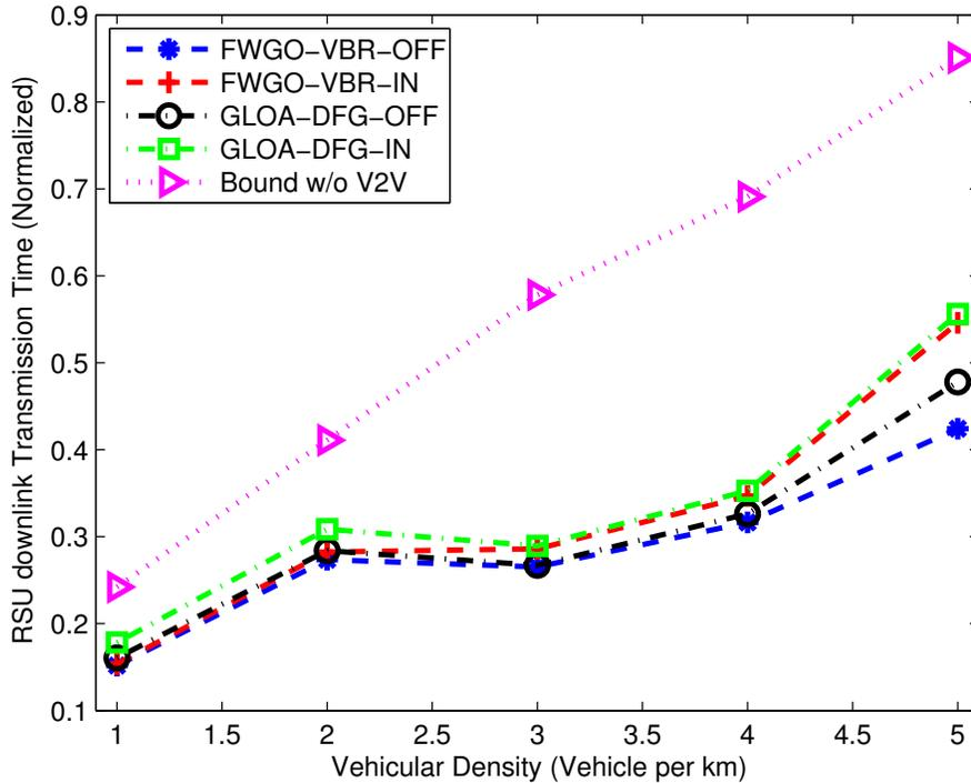
Fig. 12: RSU Downlink Transmission time vs. Vehicular Density. This plot has the same parameters as Figure 10 except that vehicle speed has been taken from a Gaussian distribution with a mean 20 m/s and a standard deviation of 2.
