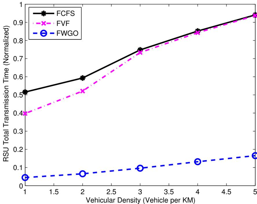
Fig. 17: RSU Downlink Transmission Time vs. Vehicular Density. All vehicles have the same job size of 3 (in terms of maximum bit rate). Vehicle speeds follow a Normal distribution with a mean of 20 m/s and a standard deviation of 3.
