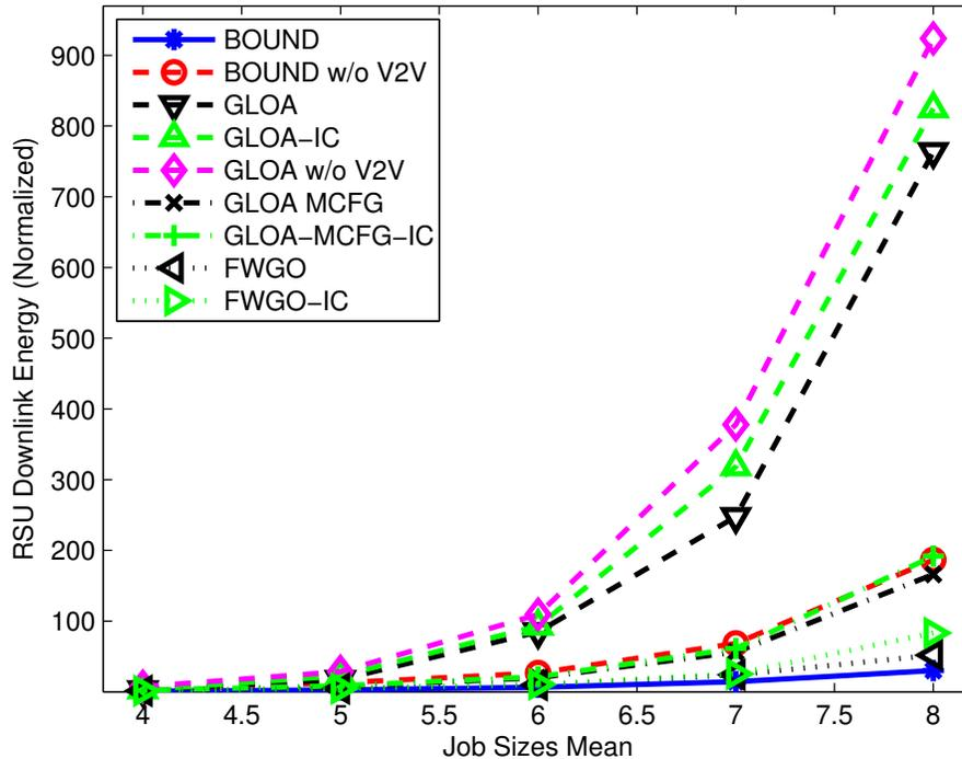
Fig. 7: Total RSU Downlink Energy vs. Job Sizes Mean. Vehicular Density is constant and equal to 4 vehicles per km, the job sizes are from a Gaussian distribution with Standard Deviation of 2
