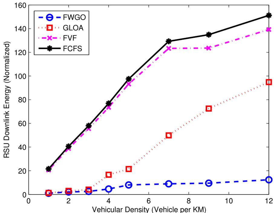
Fig. 13: RSU Downlink Energy (Normalized) vs. Vehicular Density. Vehicle job size is taken from a Normal distribution with a mean of 5 and a standard deviation of 2. Vehicle speeds follow a Normal distribution with a mean of 20 m/s and a standard deviation of 2.
