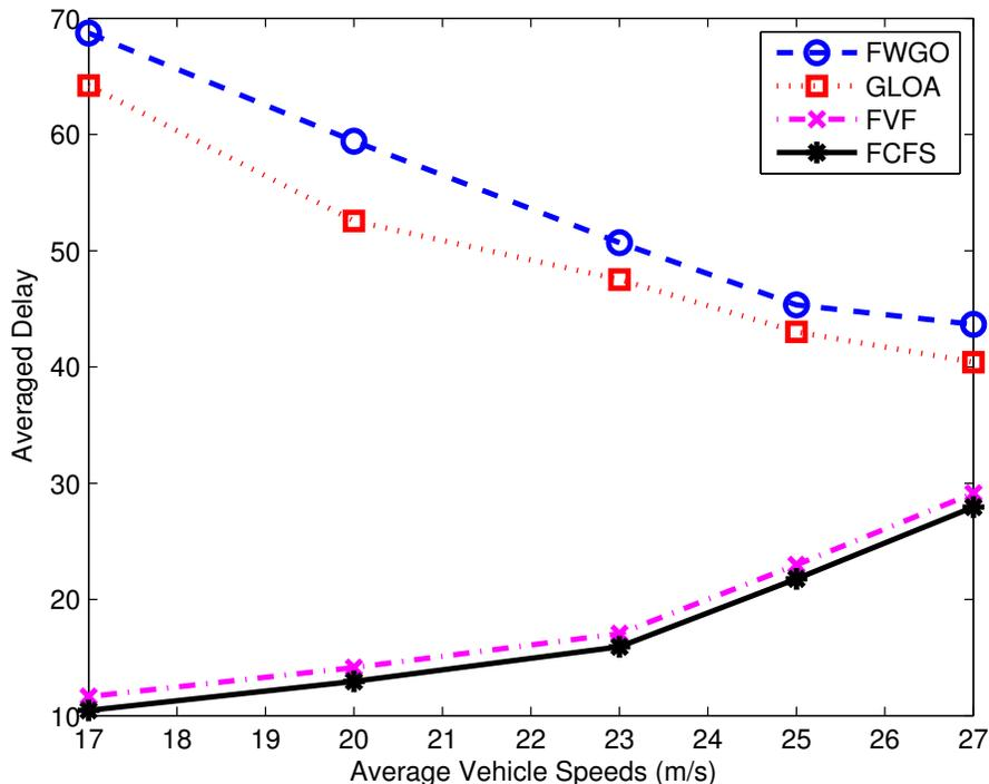
Fig. 16: Average Delay vs. Average Vehicle Speed (m/s). Vehicular density is 5 (v/km). Vehicle job size is taken from a Normal distribution with a mean of 7 and a standard deviation of 2. Vehicle speeds follow a Normal distribution with a mean shown on the x-axis and a standard deviation of 2.
