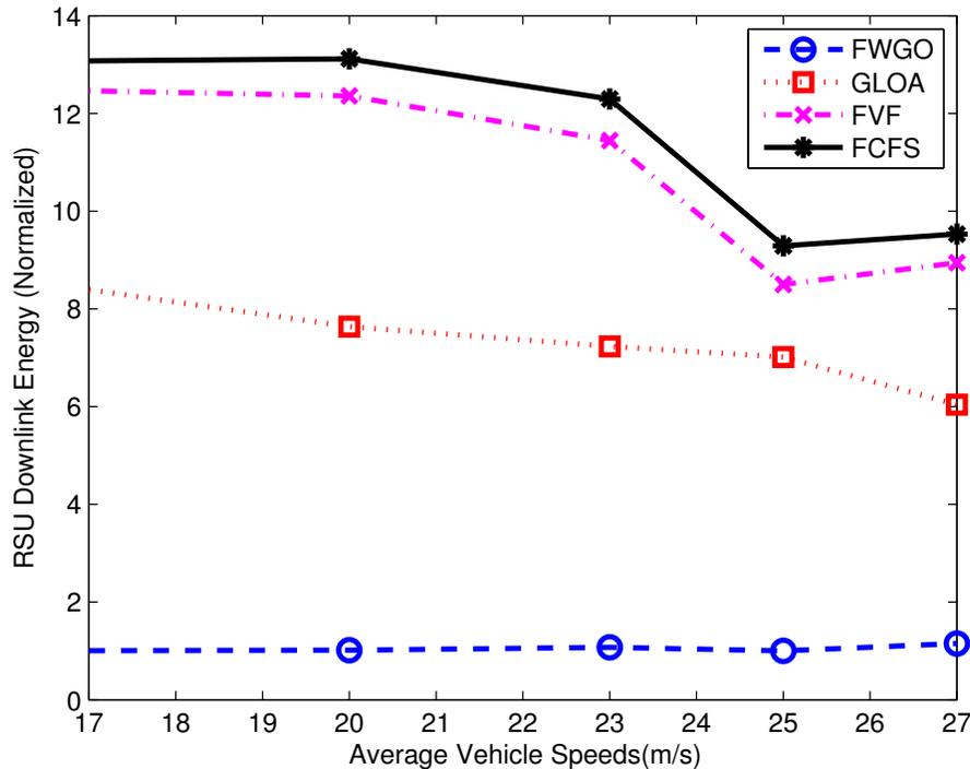
Fig. 15: RSU Downlink Energy (Normalized) vs. Average Vehicle Speed (m/s). Vehicular density of 5 (v/km). Vehicle job size is taken from a Normal distribution with a mean of 7 and a standard deviation of 2. Vehicle speeds follow a Normal distribution with a mean shown on the x-axis and a standard deviation of 2.
