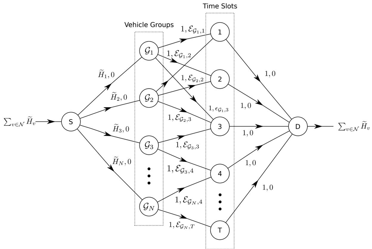
Fig. 4: Minimum Energy Vehicle Group Flow Graph Scheduler. Each edge is labeled with an ordered pair,  $(u_{i,t}, c_{i,t})$ , where  $u_{i,t}$  and  $c_{i,t}$  are the capacity and cost of using edge  $(i, t)$ . The input and output nodes,  $I$  to  $O$ , carry a flow of  $\sum_{v \in \mathcal{N}} \tilde{H}_v$ . They are connected to the rest of the graph by zero cost edges.
