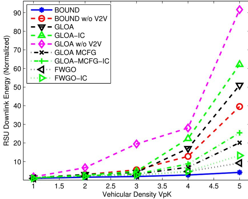
Fig. 5: Total RSU Downlink Energy vs. Vehicular Density (Vehicle per km). Speed is constant and equal to 20 m/sec for all the vehicles. The job sizes were taken from a Gaussian distribution with a mean of 5 and a standard deviation of 2.
