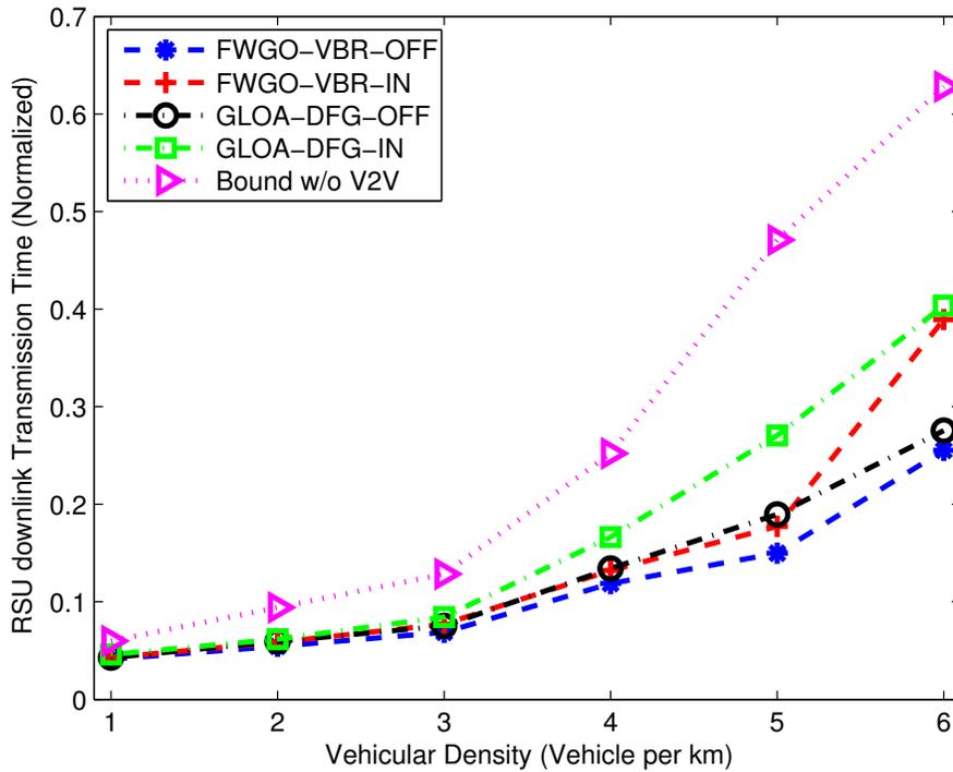
Fig. 10: RSU Downlink Transmission Time vs. Vehicular Density. Vehicle demand is taken such that 85% of vehicles have no job, but the rest have a demand of 15 time slots. The vehicle speeds are all 20 m/s.
