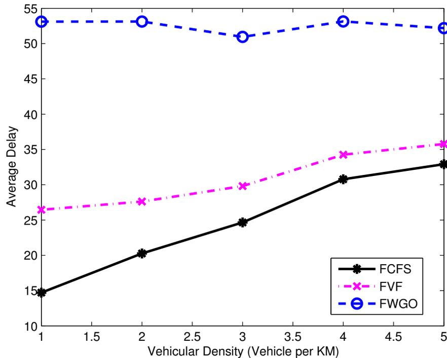
Fig. 18: RSU Downlink Transmission Time vs. Vehicular Density. All vehicles have the same job size of 3 (in terms of maximum bit rate). Vehicle speeds follow a Normal distribution with a mean of 20 m/s and a standard deviation of 3.
