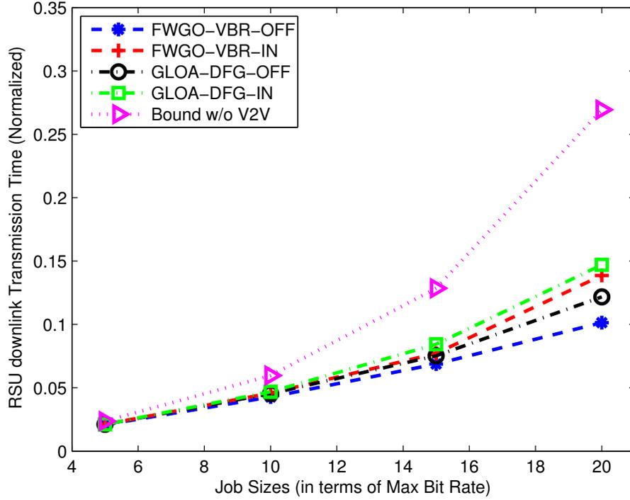
Fig. 11: RSU Downlink Transmission Time vs. Vehicle Job Demand. This graph uses the same parameters as in Figure 10 except that the high vehicle demands are varied. Vehicular density is 4/km.
