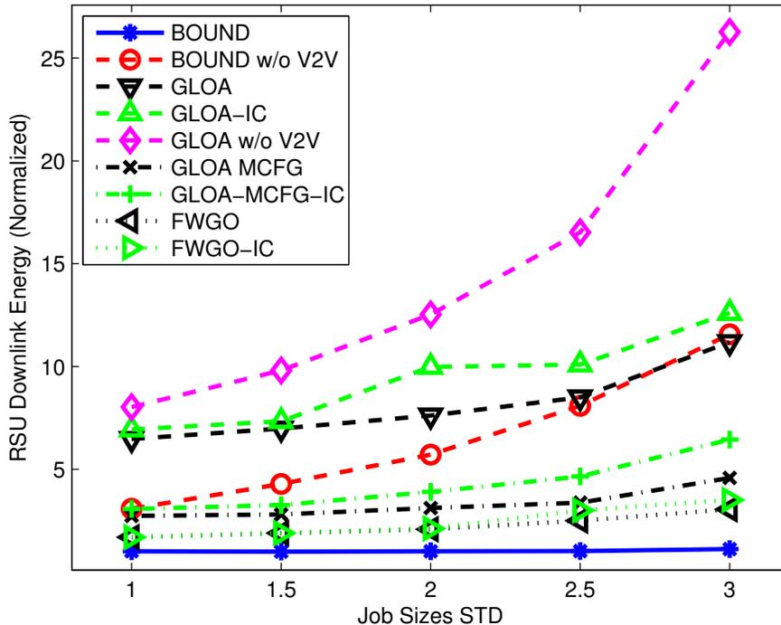
Fig. 8: Total RSU Downlink Energy vs. Job Size Standard Deviation. The mean job size is constant and equal to 5. Vehicular density is constant and equal to 4 vehicles per km and vehicle speed is constant and equal to 20 m/sec.
