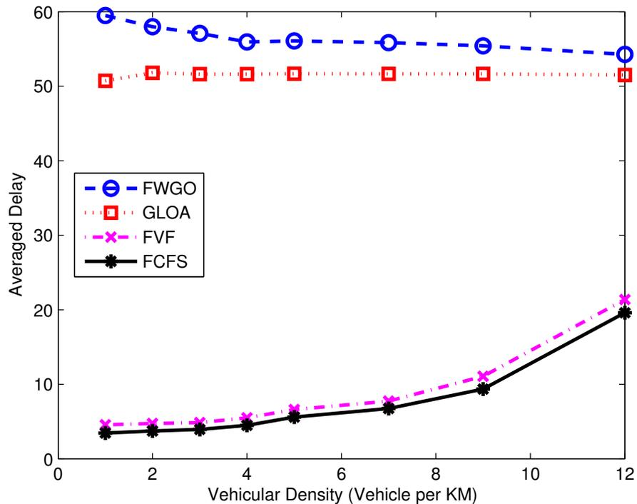
Fig. 14: Average Delay vs. Vehicular Density. Vehicle job size is taken from a Normal distribution with a mean of 5 slots and a standard deviation of 2. Vehicle speeds are from a Normal distribution with a mean of 20 m/s and a standard deviation of 2.
