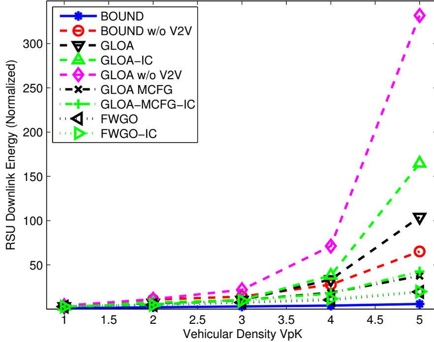
Fig. 9: Total RSU Downlink Energy vs. Vehicular Density (Vehicle per km). This plot has the same assumptions as Figure 5 but including log-normal shadowing with a zero mean and a standard deviation of  $\sigma = 4$  dB.
