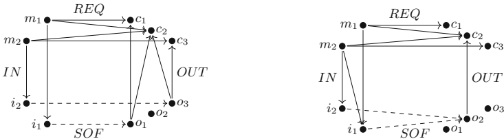
(a) REQ is implementable, but not strongly controllable (b) REQ is implementable, but not strongly observable
