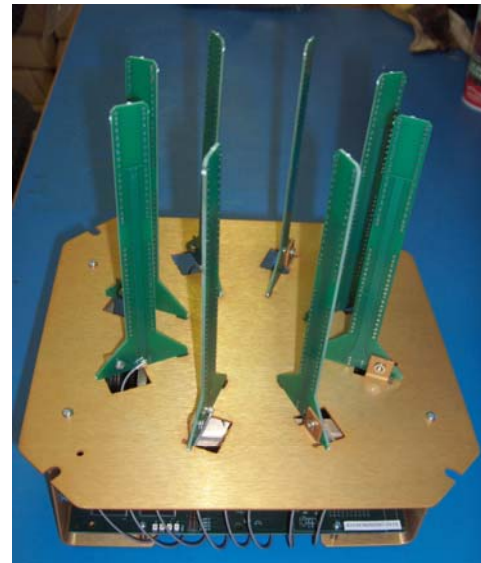
Phased-array antenna system from Fidelity Comtech
