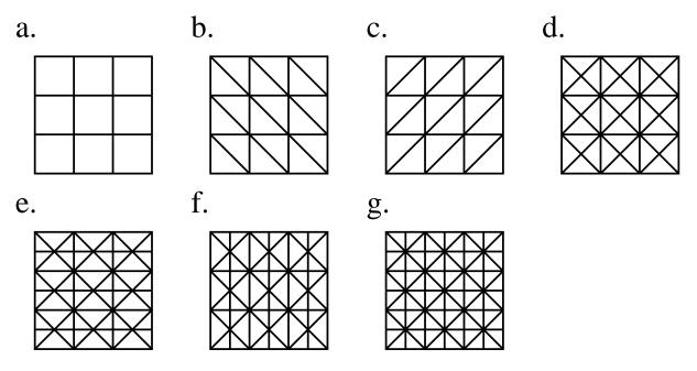
Figure 3: Parameters of variation for patterns for structured mesh discretizations
