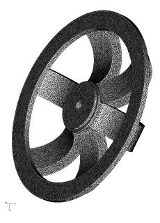
Figure 2: Example unstructured finite element mesh by P. Lefèvre
