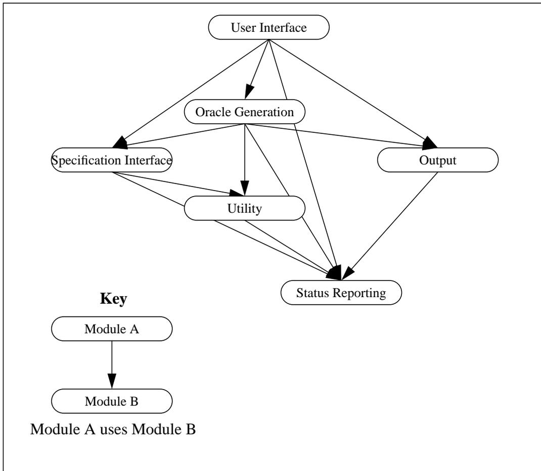
**FIGURE 2 - First Level Decomposition Module Uses Relation**
