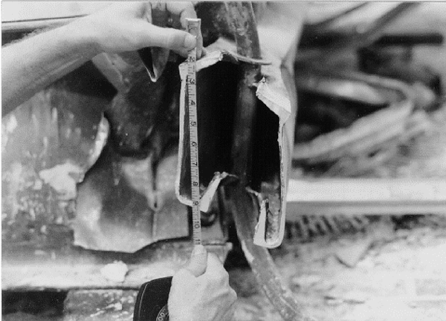
Figure 5: Connection box deformation [6]
