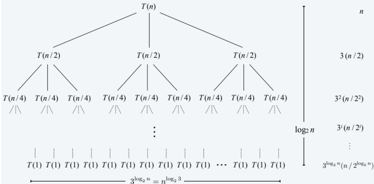
$$r = 3/2 > 1 \quad T(n) = (1 + r + r^2 + r^3 + \dots + r^{\log_2 n}) n = \frac{r^{1+\log_2 n} - 1}{r - 1} n = 3n^{\log_2 3} - 2n$$
