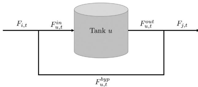
Fig. 2. Model of buffer tank  $u$ , with  $i \in I_u$ ,  $j \in J_u$ .
