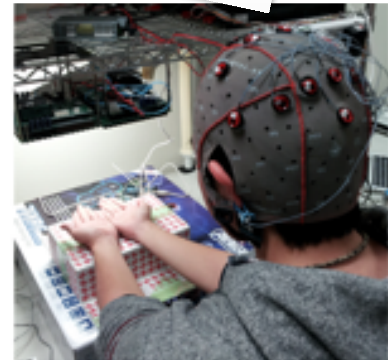
The user during autdBCI experiment with the both palms placed under the AUTD array with ultrasonic transducers.
