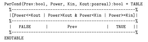
Figure 2: PVS Specification of general PwrCond function
