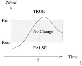
The figure to the left illustrates a power conditioning function that is used in an industrial control system. When the Power level drops below Kout, a sensor becomes unreliable so it is "conditioned out" by setting PwrCond to FALSE. When the power exceeds Kin, the sensor is "conditioned in" and is used to evaluate the system. While Power is between Kout and Kin, the value of PowerCond is left unchanged by setting it to its previous value, Prev.
