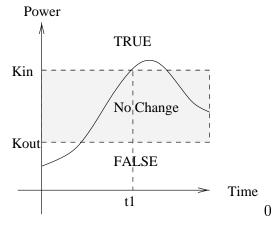
The figure to the left illustrates a power conditioning function that is used in an industrial control system. When the Power level drops below Kout, a sensor becomes unreliable so it is "conditioned out" by setting PwrCond to FALSE. When the power exceeds Kin, the sensor is "conditioned in" and is used to evaluate the system. While Power is between Kout and Kin, the value of PwrCond is left unchanged by setting it to its previous value, Prev.
