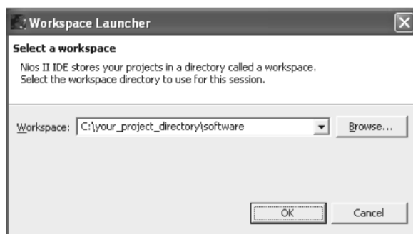
Figure 16.1 Setting the Nios II IDE workspace to the Nios II reference design software directory.
