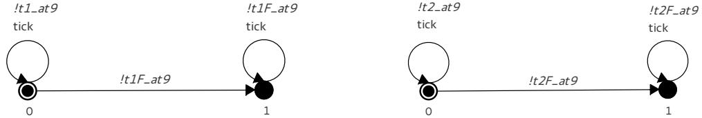
Figure 15.39: Sensor 9 and Train 1 with Figure 15.40: Sensors 9 and Train 2 with Permanent Faults
