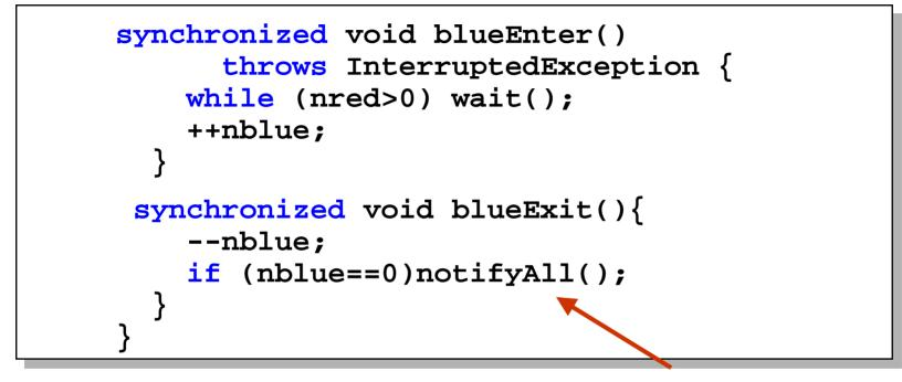
To avoid unnecessary thread switches, we use *conditional notification* to wake up waiting threads only when the number of cars on the bridge is zero i.e. when the last car leaves the bridge.
