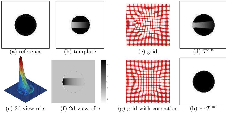
**Fig. 1.** Academic example: (a) disk as reference, (b) smaller disk with ramp as template, (c) deformed grid (no grayscale correction), (d) deformed template (no grayscale correction), (e) 3d and (f) 2d visualizations of the homogenization correction, (f) deformed grid (with grayscale correction), (g) deformed and corrected template.
