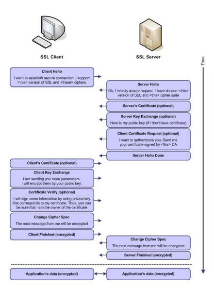
Fig. 1. SSL connection setup
