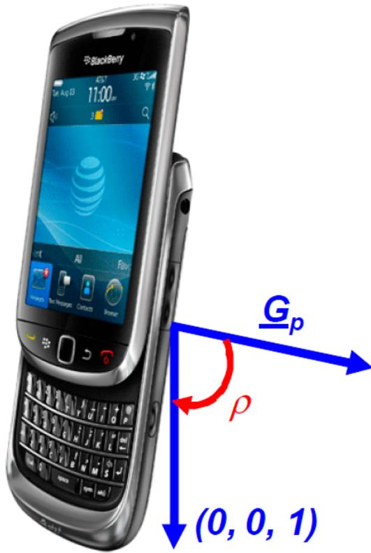
If the accelerometer reading is  $G_p$ , then in the absence of linear acceleration:
