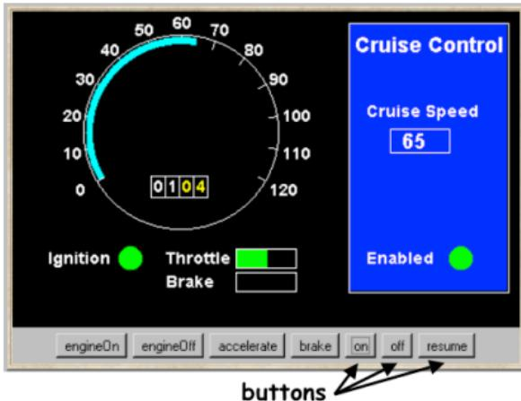
When the car ignition is switched on and the *on* button is pressed, the current speed is recorded and the system is enabled; it maintains the speed of the car at the recorded setting. Pressing the *brake*, *accelerator* or *off* button disables the system. Pressing *resume* enables the system.
