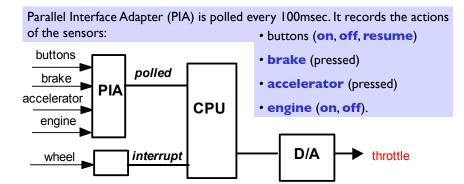
Wheel revolution sensor generates interrupts to enable the car **speed** to be calculated.
