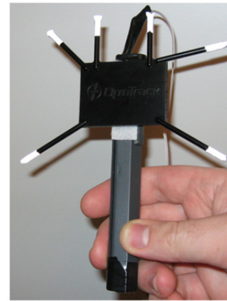
Figure 2. Tracked pen used. The button is under the thumb in this figure.
