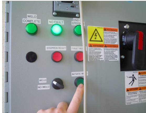
Figure 9: Turning on the resistance heating module from the Resistance heating control box to start the test.
