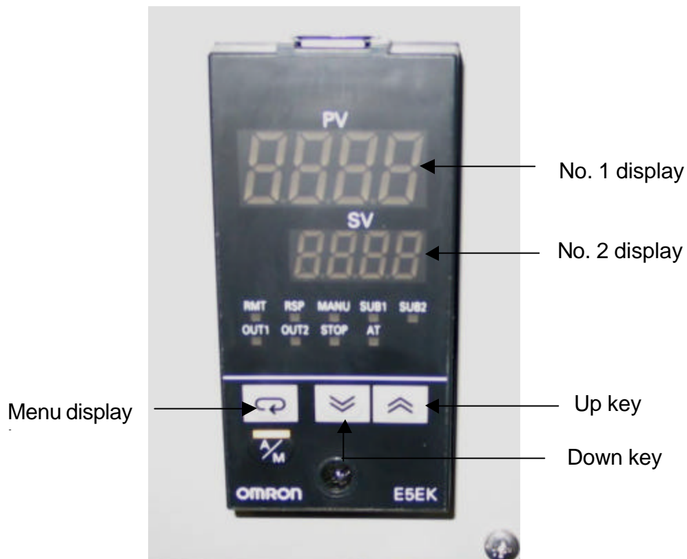
Figure 13 – Temperature controller front panel.
