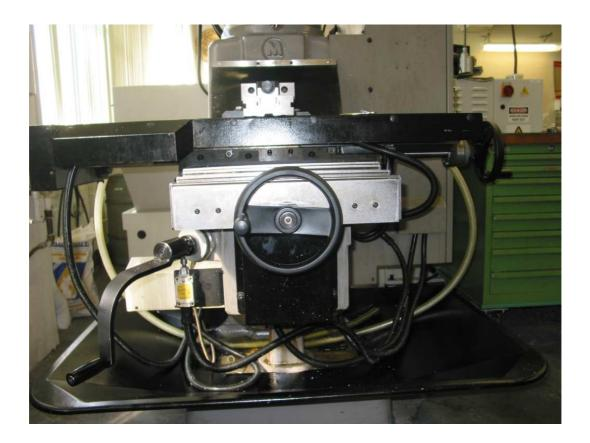
X and Z axes hand feed handles
