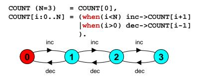
It usually occurs in the form (when  $B \times A \to P \mid when \neg B \setminus V \to Q$ ), so the choice between  $x \to P$  and  $y \to Q$  is exclusive.
