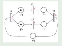
$$P = \{p_1, p_2, p_3, p_4, p_5\}, T = \{t_1, t_2, t_3, t_4\},\$$
