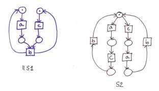
• If simultaneity is observed, the net ||S1| generate traces like  $\{a,c\} \rightarrow b \rightarrow \{a,c\} \rightarrow b \rightarrow a \rightarrow c \rightarrow \ldots$ , while S2 can only generate traces like  $a \rightarrow b \rightarrow c \rightarrow \ldots$  and  $c \rightarrow b \rightarrow c \rightarrow \ldots$
