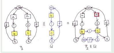
$\spadesuit$   $P_2 \parallel Q$  **deadlocks** after firing 'red' *a* and placing a token in the place 2!
