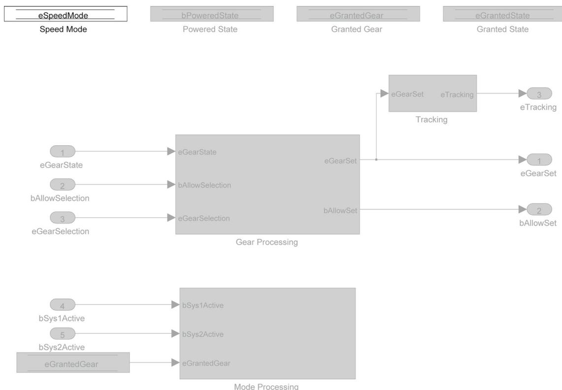
**Fig. 12** Subsystem Gear and Mode Processing after Reach and Coreach were run on all its inputs and outputs, respectively
