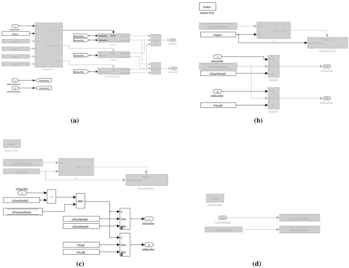
**Fig. 13** Impact analysis. **a** Reach from last four inputs of the If GearState block. **b** Effect of last four inputs of If GearState on If Gear1 only (If Gear1 subsystem). **c** Effect of last four inputs of If GearState
