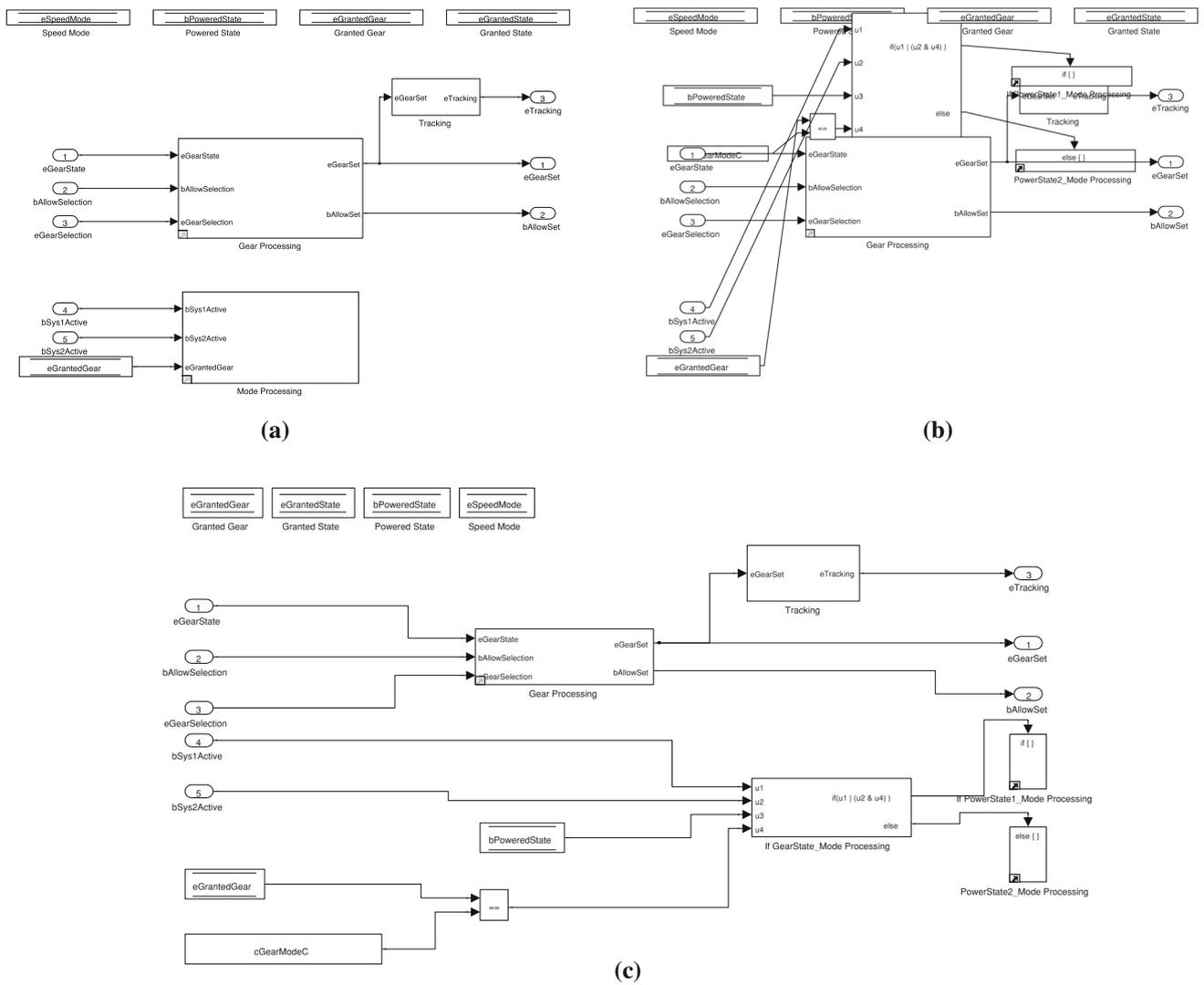
Fig. 21 Illustration of Flatten Subsystem transformation. **a** Subsystem Gear and Mode Processing before Subsystem Flatten. **b** Intermediate stage in flattening subsystem Mode Processing. **c** Subsystem Gear and Mode Processing after flattening subsystem Mode Processing
