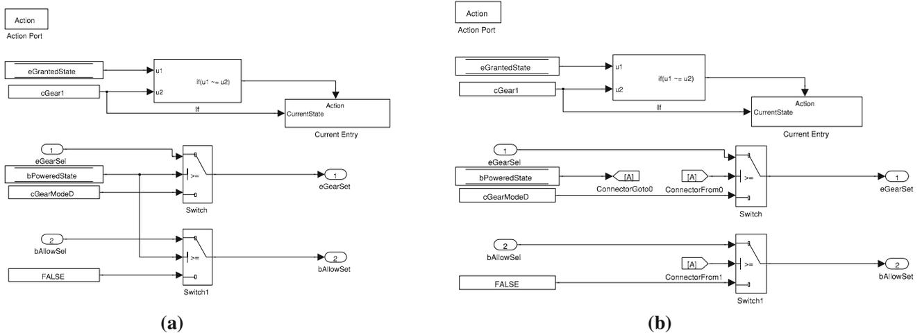
Fig. 20 Illustration of Signal Line to Goto/From transformation. **a** Before. **b** After
