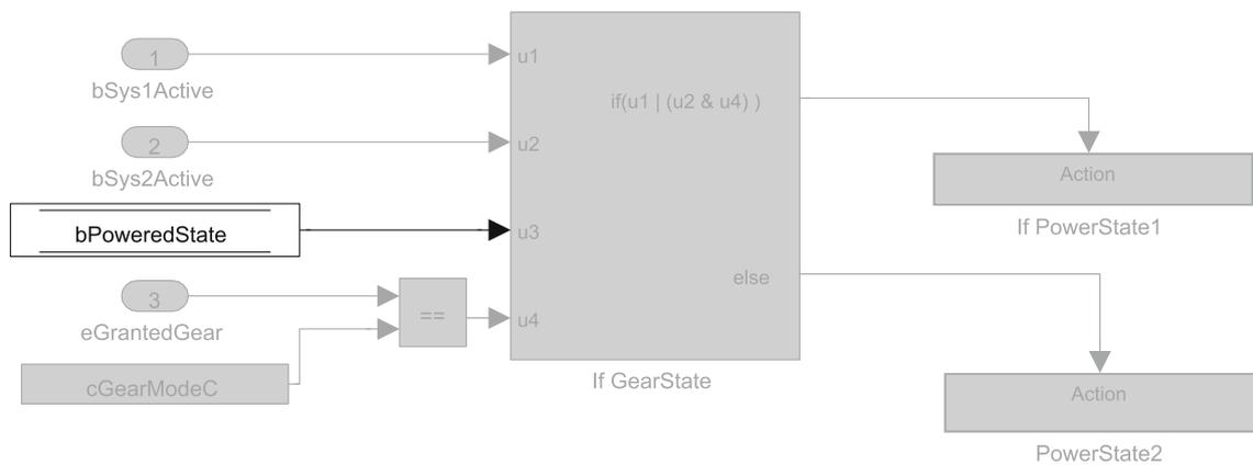
**Fig. 11** Subsystem Mode Processing after Coreach was run on all outputs of Gear and Mode Processing
