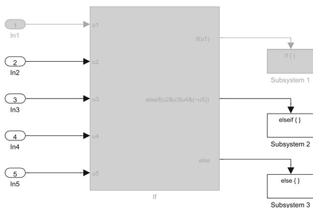
**Fig. 10** Coreach on Subsystem 1: first output of If block is affected by first input only
