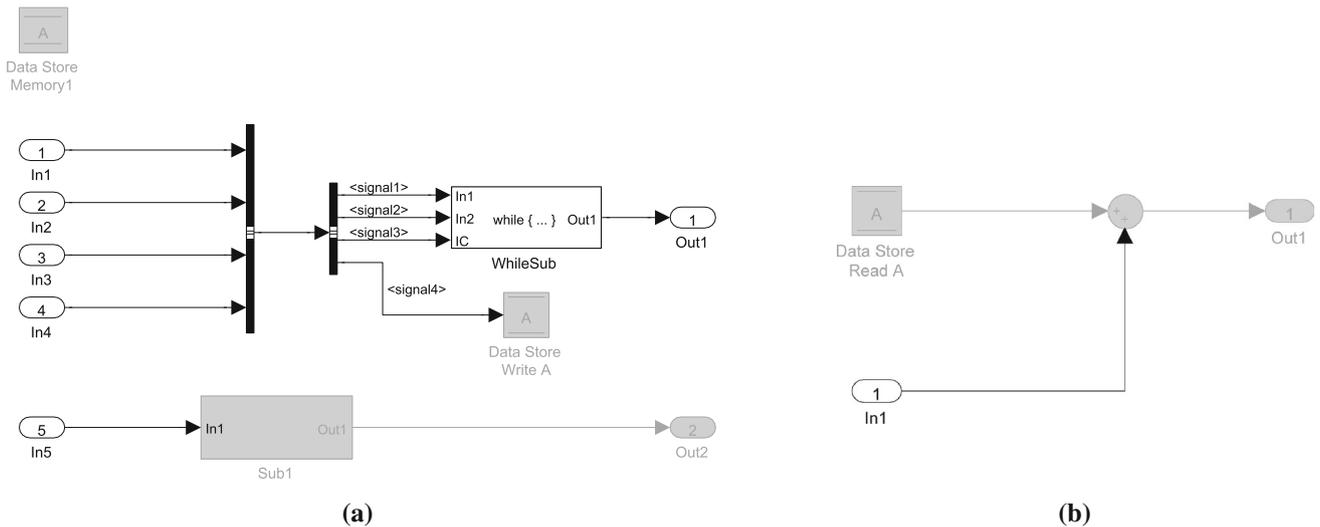
**Fig. 9** Reach analysis for Data Store Write A. **a** Reach for Data Store Write A. **b** Subsystem Sub1 from **a**
