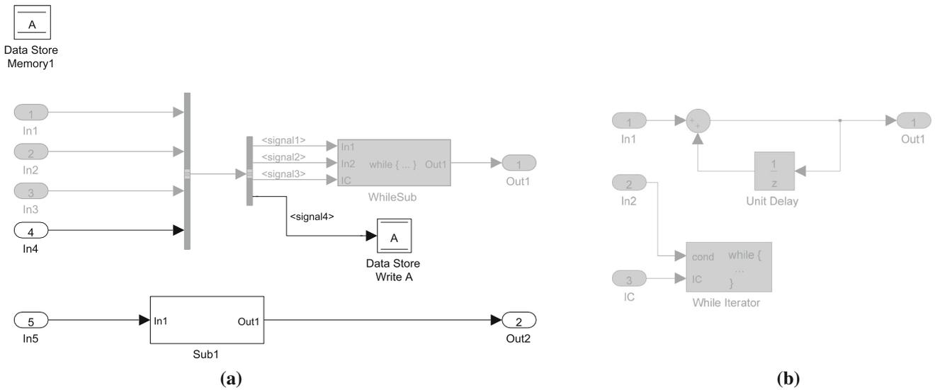
**Fig. 8** Coreach analysis for Out1. **a** Coreach for Out1. **b** Subsystem WhileSub from **a**
