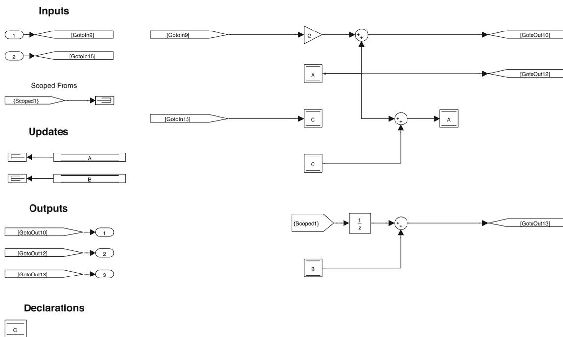
Fig. 5 Subsystem Sub1 including weak signature generated by the Signature Tool
